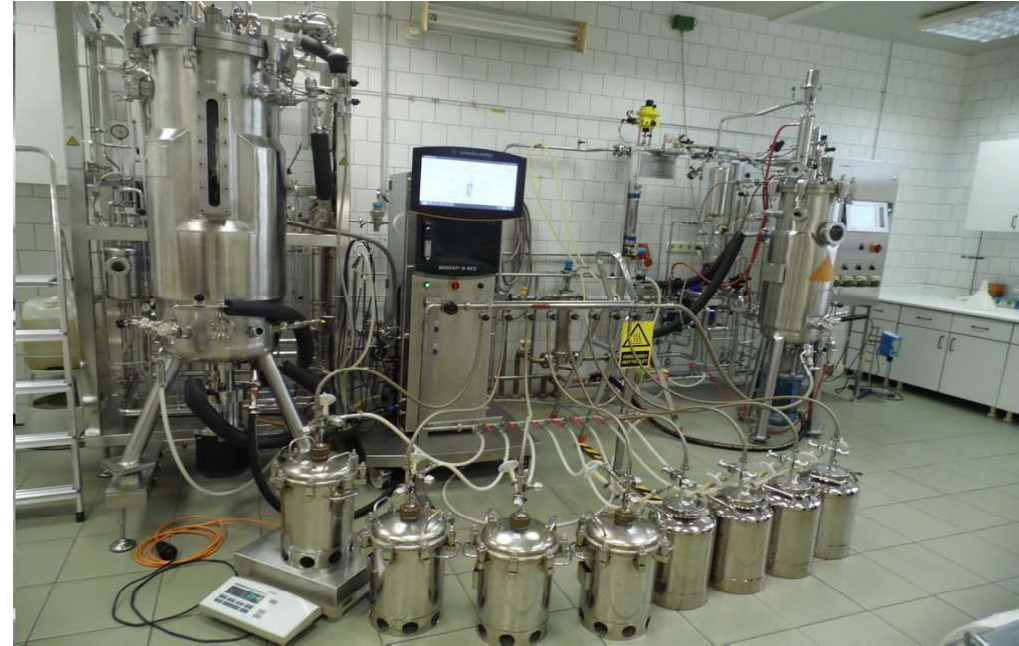
Inoculum fermentation for production in 75 and 150 liter fermenters
