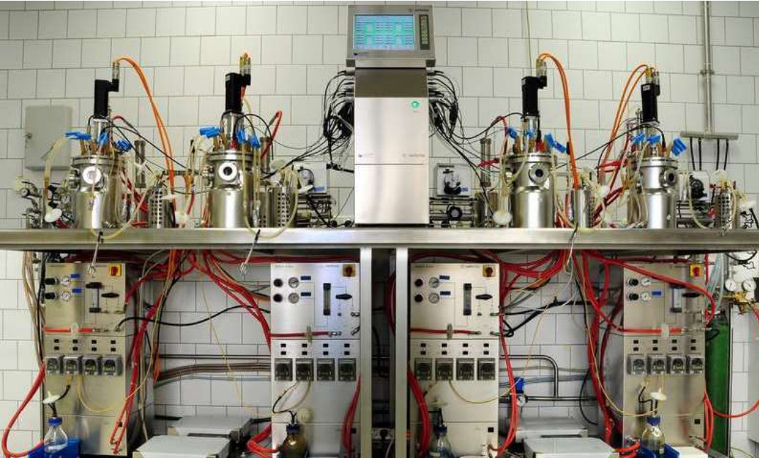
2 liter fermenters for raw material tests and process optimization trials
